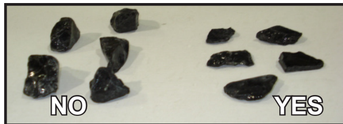
Figure 1. Selecting Flat Rocks for Pilot Cover
